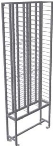
These minimal footprint floor mounted racks are designed to protect masks from particulation and ESD. Special structure enables clean air to flow through rack and keep particles off. Each mask is seated in a separate port. This product can be modified according to mask type. An enclosed version with doors is also available. Fabrication material: 304 stainless steel, electropolished.
